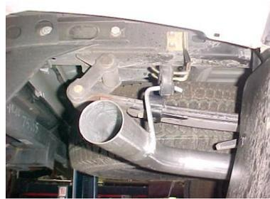
INSTALL WELDED HANGER INTO GROMMET.
