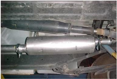
THEN INSTALL THE MUFFLER ON HEADPIPE #A NO LESS THAN 1-1/2" TO 2" USING CLAMP #E. THE MUFFLER OUTLET WILL BE Clocked AT 12 O'CLOCK POSITION. INLET OF MUFFLER HAS LOUVERS FACING THE MOTOR. DO NOT TIGHTEN.
