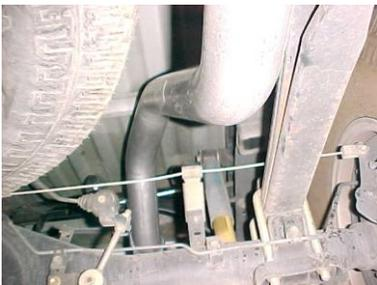
INSTALL THE STAINLESS TIP. USE A STAINLESS STEEL OR ALUMINUM CLEANER AND ANY SCOTCH BRITE PAD TO CLEAN. NOW TIGHTEN ALL HANGERS AND CLAMPS.
