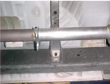
SLIDE THE HEADPIPE ONTO THE STOCK HEADPIPE ATTACHING CLAMP # E.
