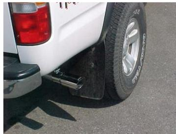
**MAKE SURE YOU HAVE A MINIMUM OF A 1" CLEARANCE FROM ALL BRAKE LINES, FUEL LINES, TIRES, SHOCKS, ETC...**
