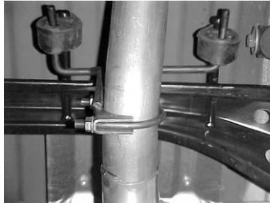
INSTALL REAR MUFFLER HANGER #C TO SUPPORT THE TAILPIPE. THE BOLTS FROM THE OE HANGER WILL BE FACING THE DRIVERSIDE. THIS HANGER ATTACHES TO THE TAILPIPE, NOT THE MUFFLER. DO NOT TIGHTEN.
