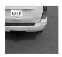
INSTALL YOUR STAINLESS STEEL TIP. USE ANY ALUMINUM OR STAINLESS STEEL CLEANER TO POLISH YOUR TIP. CHECK ALL YOUR CLEARANCES AND TIGHTEN ALL CLAMPS AND HANGERS.
