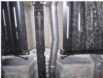
4. Slide intermediate pipe #B over headpipe. Use clamp #G to secure. Do not tighten.
