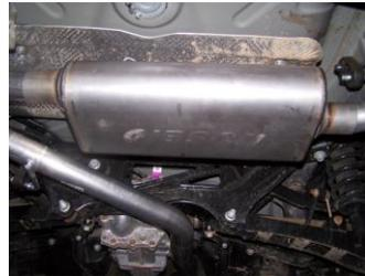
6. Slide muffler #D over inlet pipe 1.5-2". Secure with clamp #G. Do not tighten.
