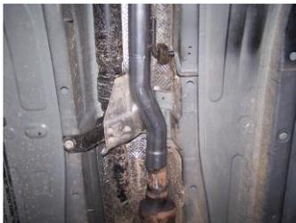
3. Slide headpipe #A over stock pipe. Secure using clamp #G. Do not tighten. Use a jack stand to support the converter. Insert welded hanger into rubber grommet.
