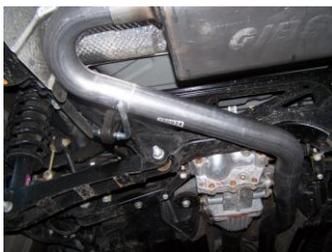
5. Slide inlet pipe #C over the intermediate pipe. Insert welded hanger into rubber grommet. Secure with clamp #G. Do not tighten.
