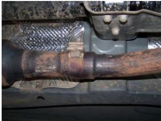
2. To remove your stock exhaust, unclamp it after the catalytic converter. Disengage the welded hangers from the rubber grommets. Use WD-40 to aid in this process. Do not damage or remove the rubber grommets as you will reuse them to mount your new system.
