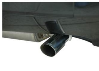
8. Install stainless steel tip. Clamp down. When you have everything in place, firmly tighten all clamps down securely. Use stainless steel cleaner and a Scotch Brite pad weekly to prevent tip from discoloration. Inspect all fasteners after 25-50 miles of operation and re-tighten as necessary.
