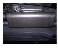
Install muffler #B onto head pipe #A  $1\frac{1}{2}$ -2" with the louvers facing towards the converter. Use a jack stand to support the muffler. Use clamp #E to secure the muffler to the head pipe. DO NOT TIGHTEN. Muffler inlet is looking into the louvers.
