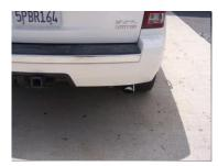
When you have everything in place, firmly tighten all bolts and clamps down securely. To clean stainless steel tips, use stainless steel cleaner and a Scotch Brite pad.
