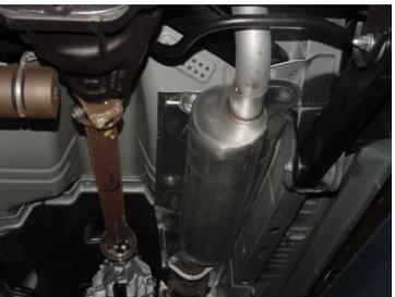
INSTALL MUFFLER #B 1-1/2" TO 2" ONTO THE HEADPIPE WITH INLET FACING TOWARDS THE MOTOR. ROTATE THE MUFFLER UNTIL THE OUTLET IS AT THE 2 O'CLOCK POSITION. USE CLAMP #E TO SECURE THE MUFFLER TO THE HEADPIPE. MUFFLER INLET IS LOOKING INTO THE LOUVERS. DO NOT TIGHTEN.
