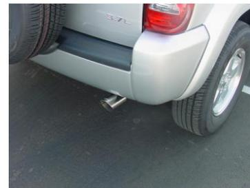
INSTALL THE STAINLESS STEEL TIP. TO CLEAN TIP USE A SCOTCH BRITE PAD AND ANY STAINLESS OR ALUMINUM CLEANER. NOW GO BACK AND TIGHTEN ALL CLAMPS, NUTS AND BOLTS STARTING FROM THE FRONT AND WORKING BACK.
