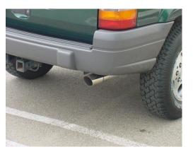
**INSTALL YOUR** STAINLESS TIP TO YOUR DESIRED LOOK. TO CLEAN TIP USE ANY ALUMINUM OR STAINLESS CLEANER AND A SCOTCH BRITE PAD. NOW TIGHTEN ALL CLAMPS STARTING FROM THE FRONT AND WORKING BACK.
