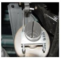
USE HANGER #F AT THE REAR OF THE MUFFLER WITH VERTICAL BAR OF HANGER ON PASSENGER SIDEAND INSERT WELDED ROD INTO RUBBER GROMMET. DO NOT TIGHTEN.
