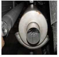
SLIDE MUFFLER WITH BAFFLES FACING FORWARD TOWARDS CONVERTER ONTO THE HEADPIPE NO LESS THEN 1½" AND NO MORE THAN 2". MUFFLER INLET IS LOOKING INTO LOUVERS.
