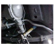
Install the overaxle tailpipe #B. Attach to muffler with hanger #D, Insert welded hanger into factory rubber grommet.
