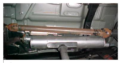
3. INSTALL THE MUFFLER # A TO THE STOCK FLANGE USING BOLT KIT # F AND GASKET # E WE SUGGEST USING A HIGH TEMP GASKET SEALER ON THE STOCK GASKET WHEN REINSTALLING. USE JACKSTANDS TO SUPPORT THE MUFFLER. INSTALL HANGER #D IN REAR RUBBER GROMMETS NEAR THE OUTLET OF THE MUFFLER.
