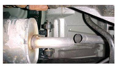
1. NOW, CUT STOCK TAILPIPE JUST ABOVE THE FIRST BEND COMING OUT OF THE REAR OF THE STOCK MUFFLER. REMOVE STOCK TAILPIPE.
