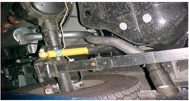
4. INSTALL TAILPIPE #B AND INSERT WELDED HANGER INTO RUBBER GROMMETS AND THEN INSERT IT INTO THE REAR OF THE MUFFLER. AND ATTACH WITH HANGER #D. INSTALL THE STAINLESS TIP. TO CLEAN USE ANY STAINLESS OR ALUMINUM CLEANER..
