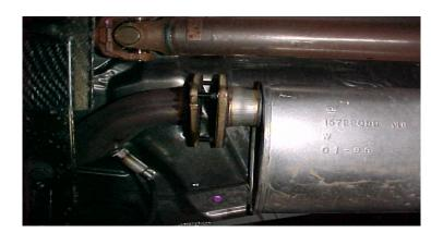
2. UNBOLT STOCK MUFFLER FLANGE AT THE STOCK CONVERTER. REMOVE THE STOCK MUFFLER. MAKE SURE ALL RUBBER GROMMETS ARE STILL IN PLACE.
