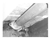
TO REMOVE STOCK EXHAUST UN-BOLT IT FROM THE 2-BOLT FLANGE LOCATED BETWEEN THE CATALYTIC CONVERTER AND THE MUFFLER. NOW CUT OFF YOUR STOCK TAILPIPE JUST BEHIND THE MUFFLER AND REMOVE. LEAVE ALL RUBBER GROMMETS ON THE HANGER. USE WD-40 TO AID IN REMOVAL OF EXHAUST AND HANGERS. INSTALL HEADPIPE #A, USE # G GASKET, AND RE-USE YOUR FACTORY BOLTS. DO NOT TIGHTEN.
