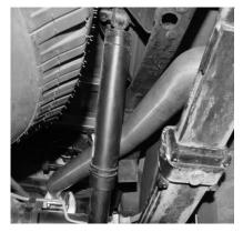
INSTALL TAILPIPE #C ONTO MUFFLER 1-1/2" TO 2". THE TAILPIPE WILL GO BETWEEN TIRE AND SHOCK, INSTALL FROM THE REAR OF THE VEHICLE. INSERT WELDED HANGER INTO THE RUBBER GROMMET. AND ATTACH WITH HANGER # E.
