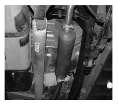
INSTALL MUFFLER #B ONTO HEADPIPE 1-1/2" TO 2" WITH INLET TOWARDS THE ENGINE. OUTLET SHOULD BE AT THE 12 O'CLOCK POSITION. USE CLAMP #F TO SECURE MUFFLER TO THE HEADPIPE, DO NOT TIGHTEN. THE INLET OF THE MUFFLER IS LOOKING INTO THE LOUVERS.
