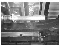
REMOVE STOCK EXHAUST BY UNBOLTING IT FROM THE 2 BOLT FLANGE JUST IN FRONT OF THE CONVERTER. DO NOT REMOVE STOCK STUDS. LEAVE ALL RUBBER GROMMETS IN THE STOCK POSITION. USE WD-40 TO AID YOU IN REMOVING THE RUBBER GROMMETS FROM THE STOCK HANGERS. FOR EASIER REMOVAL CUT THE TAILPIPE JUST BEHIND THE MUFFLER.
