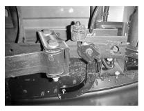
REMOVE FACTORY REAR TAILPIPE EXHAUST HANGER FROM FRAME.
