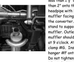
3. Slide muffler #B no less than 1½" and no more than 2" onto the front headpipe with louvers in muffler facing towards the converter. Use a jack stand to support the muffler. Outlet of muffler should be clocked at 9 o'clock. Attach using clamp #G. Install rear hanger #F onto muffler. Do not tighten. Muffler inlet is looking into the louvers.
