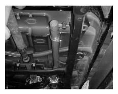
2. Bolt on front headpipe #A using bolt kit #I and gasket #H. Use a RTV gasket sealer for flange connection. (Note Headpipe will lean toward passenger side.)
