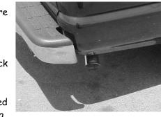
5. Install stainless steel tip. Clamp down. To clean stainless steel tip use any stainless or aluminum cleaner. When you have everything in place, tighten all bolts and clamps.
