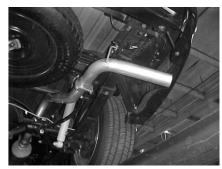
INSTALLING OVERAXLE TAILPIPE. YOU MUST UNBOLT FACTORY REAR TAILPIPE HANGER AND ROTATE IT 180 **DEGREES**. Insert the overaxle tailpipe. #C no less than  $1\frac{1}{2}$  and no more than 2". Slightly lean to the driver side. Slide turnout pipe #D on to the tailpipe. Roll turnout pipe until you have it at the correct angle for your truck. Insert welded hanger into rubber grommet. Clamp down. Using clamp #G
