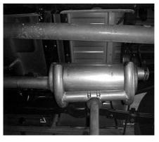
1. Lay out the GIBSON EXHAUST SYSTEM on the floor so it looks like the drawing. Match all part numbers with the manual. Unbolt stock exhaust from behind the catalytic converter. Leave all rubber grommets in place. Use jack stands to support converter. You will re-use the factory nuts on headpipe flange.
