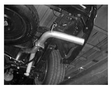
4. BEFORE INSTALLING OVERAXLE TAILPIPE, THE FACTORY REAR TAILPIPE HANGER MUST BE UNBOLTED AND ROTATED 180 DEGREES. Insert the overaxle tailpipe. #C no less than  $1\frac{1}{2}$  and no more than 2". Slightly lean to the driver side. Slide turnout pipe #D on to the tailpipe. Roll turnout pipe until you have it at the correct angle for your truck. Insert welded hanger into rubber grommet. Clamp down. Using clamp #H
