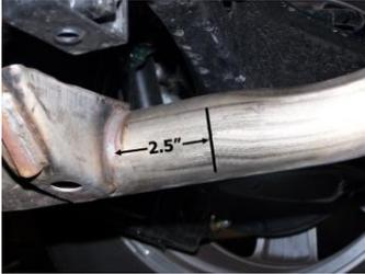
2. To remove stock exhaust, measure 2.5" from exhaust hanger located before the 2-bolt flange. See picture. Remove stock exhaust from the 3 rubber hangers. Use WD-40 to aid in removal.
