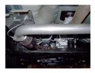
3. Install headpipe #A onto the existing stock flange and attach with the factory nuts. Re-attach the ground strap. Do not tighten the nuts.
