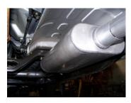
5. Install muffler #C onto headpipe #B 1.5-2" with the louvers facing towards the converter. Use a jack stand to support the muffler. Use clamp #G to secure the muffler to the headpipe. Do not tighten. Muffler inlet is looking into the louvers.
