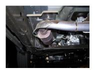
2. First remove the clamp behind your factory muffler. Now remove the tailpipe. Now unbolt the 2-bolt and remove the rest of your exhaust system. Save your factory nuts as you will re-use them.
