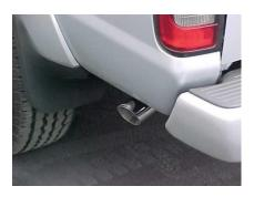
NEXT INSTALL YOUR STAINLESS STEEL TIP TO YOUR DESIRED LOOK. USE A STAINLESS OR ALUMINUM CLEANER TO POLISH TIP. NOW TIGHTEN ALL CLAMPS STARTING FROM THE FRONT AND WORKING BACK.
