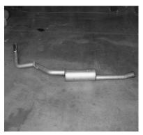
LAY OUT THE GIBSON EXHAUST ON THE FLOOR AND COMPARE PART NUMBERS WITH THE MANUAL. LEAVE ALL FACTORY GROMMETS IN PLACE. FOR EASIER REMOVAL OF GROMMETS AND HANGERS USE WD-40 ON THEM.
