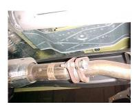
Unbolt stock exhaust at flange behind the catalytic converter and remove stock exhaust. Do not damage the factory gasket and bolts, you will re-use them. Use WD-40 for easier removal on all rubber grommets. Leave all stock rubber grommets in place. Slide flange #H onto Gibson head pipe #A and install head pipe to stock flange, re-use factory gasket and
