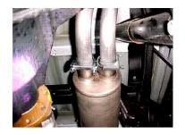
Clamps on muffler outlets should be positioned at 9 o'clock and 3 o'clock.
