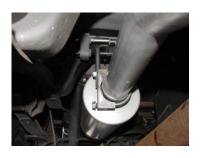
Install T-Hanger #E into factory rubber grommets in front of the muffler. **Do not tighten**
