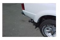
Install stainless steel tips. To clean, use a stainless or aluminum cleaner. Now tighten all clamps and hangers.
