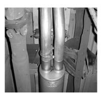
THEN, INSTALL DRIVERSIDE TAILPIPE #D. SUPPORT THE MUFFLER WITH A JACK STAND. THEN INSTALL PASSENGER SIDE OVERAXLE #C. INSERT WELDED HANGER ON TAILPIPE INTO FACTORY RUBBER GROMMENT.
