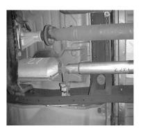
LAYOUT THE GIBSON EXHAUST SYSTEM ON THE FLOOR SO IT LOOKS LIKE THE DRAWING. THEN REMOVE THE STOCK EXHAUST SYSTEM, BUT LEAVE ALL RUBBER GROMMENTS IN PLACE. START WITH INSTALLING HEADPIPE #A ONTO CATALYTIC CONVERTER AND CLAMP #G. **DO NOT TIGHTEN!**
