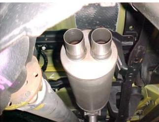
Install muffler #B onto head pipe 1-1/2" to 2" with the louvers facing towards the converter. Use a jack stand to support the muffler. Use hanger # F to the secure the muffler to the head pipe. Do not tighten. hanger #F also has a hanger welded to it. Insert into rubber grommets located above muffler inlet.
