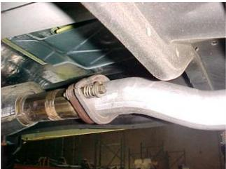
Slide flange # I onto your new head pipe #A then install head pipe #A onto you're existing stock flange using your factory hardware. Use a jack stand to support the converter.
