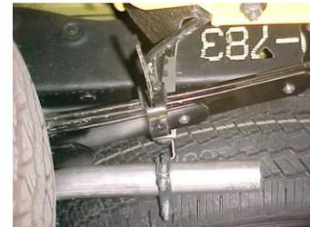
Install the passenger side tailpipe # C into the muffler at least 1-1/2" to 2". Use clamp # G to secure pipe to muffler. Do not tighten.
