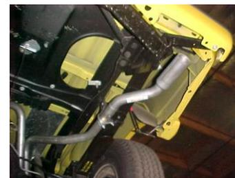
Install exit pipes # E Use clamps # G to secure exit pipes to tailpipes. Next, install you stainless tips. Now go back and tighten all clamps, nuts and bolts. Start from the front and work back. Use zip ties for brake and fuel lines.
