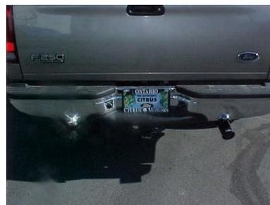
FINALLY AFTER TIGHTENING ALL CLAMPS FROM FRONT TO BACK AND MAKING SURE OF ALL CLEARANCES, INSTALL YOUR STAINLESS TIPS TO YOUR DESIRED LOOK.
