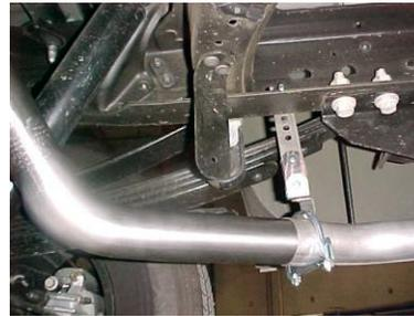
INSTALL PASSENGER SIDE OVERAXLE PIPE #C INTO MUFFLER 1 1/2" TO 2". USE CLAMP #I TO SECURE. DO NOT TIGHTEN. ROTATE UNTIL PIPE TOUCHES HANGER. #J USE CLAMP #I TO HOLD PIPE TO HANGER #J. DO NOT TIGHTEN.
