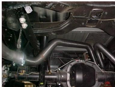
NEXT INSTALL EXIT PIPES #E ONTO OVERAXLE PIPES. USE CLAMPS #I. SECURE EXIT PIPE TO OVERAXLES.
