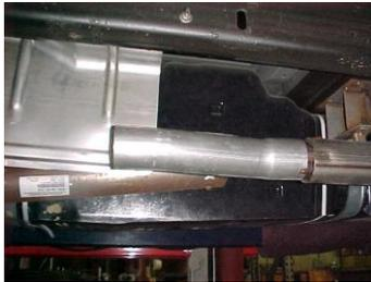
NEXT INSTALL BAND CLAMP #G. SLIDE IT OVER THE MUFFLER. THEN INSTALL HANGERS INTO THE RUBBER GROMMETS LOCATED ABOVE THE MUFFLER OUTLET. USE BOLT KIT #K TO SECURE. DO NOT TIGHTEN.
