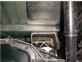
NEXT, LOCATE THE SLOTTED HOLES LOCATED APPROXIMATELY 16" FROM THE REAR OF THE FRAME. MOUNT THE 10" STRAP HANGERS #J INTO THESE SLOTS USING THE HARDWARE PROVIDED. MOUNT USING THE 2<sup>ND</sup> HOLE FROM THE TOP.
