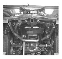
INSTALL PASSENGER SIDE OVERAXLE TAILPIPE #C INTO OUTLET OF MUFFLER. USE CLAMP #I TO SECURE, CLAMP AND SECURE THE REAR OF THE TAILPIPE TO HANGER #H USING CLAMP #I. INSTALL FRONT DRIVERSIDE OVERAXLE TAILPIPE #D AND SECURE TO MUFFLER USING CLAMP #G. **INSTALL REAR TAILPIPE #E AND SECURE TO** FRONT TAILPIPE USING CLAMP #I. CLAMP AND SECURE THE REAR OF THE TAILPIPE TO HANGER #H USING CLAMP #I. DO NOT TIGHTEN.
