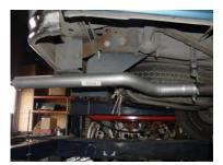
INSTALL MUFFLER #B ONTO HEADPIPE. USE A JACKSTAND TO SUPPORT THE MUFFLER. USE CLAMP #J TO SECURE THE MUFFLER TO THE HEADPIPE. DO NOT TIGHTEN.
