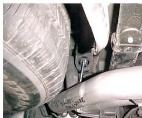
INSTALL PASS. SIDE TAILPIPE # C INTO MUFFLER 1 1/2" TO 2". INSERT HANGER INTO RUBBER GROMMET, USE CLAMP # G TO SECURE PIPE TO MUFFLER. DO NOT TIGHTEN.
