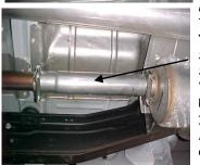
MEASURE 43" FROM THE REAR OF THE MUFFLER FORWARD AND CUT. YOU WILL BE REMOVING THE STOCK ALIGNMENT PIN. CUT STOCK EXHAUST OFF AND USE WD-40 ON ALL HANGERS. LEAVE RUBBER GROMMETS IN PLACE. INSTALL NEW HEADPIPE #A AND ATTACH TO FACTORY PIPE USING CLAMP #I.
