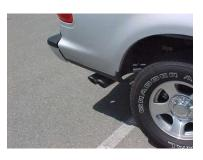
INSTALL THE STAINLESS STEEL TIPS. USE ANY ALUMINUM OR STAINLESS STEEL CLEANER TO POLISH TIP. NOW TIGHTEN ALL HANGERS AND CLAMPS.
