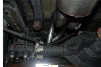
INSTALL DRIVERS SIDE TAILPIPE # D INTO MUFFLER 1 1/2" TO 2". INSERT HANGERS INTO RUBBER GROMMETS, USE CLAMP # G TO SECURE PIPE TO MUFFLER. DO NOT TIGHTEN. THE TAB ON THIS PIPE SHOULD GO ON BOTTOM OF PASSENGER SIDE PIPE USE BOLT KIT # H TO SECURE TOGETHER.
