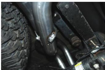
INSTALL PASS. SIDE TAILPIPE # C INTO MUFFLER 1 1/2" TO 2". INSERT HANGER INTO RUBBER GROMMET, USE CLAMP # G TO SECURE PIPE TO MUFFLER. DO NOT TIGHTEN.
