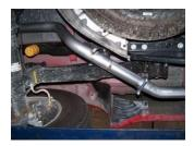
**4.** Install the passenger side overaxle tailpipe #C into the muffler  $1\frac{1}{2}$ "-2". Use clamp #Hto secure tailpipe to muffler. DO NOT TIGHTEN. Insert hanger into rubber grommet.
