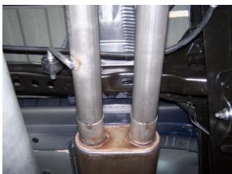
6. Install extension pipe #D into muffler. Use clamp #J to secure. Do not tighten. Next install driver side extension pipe #E into muffler using clamp #J to secure. Do not tighten. Insert welded hanger into rubber grommet.
