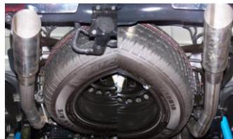
10. Next, install the exit pipes #H. Use clamps #J to secure the tailpipes.
