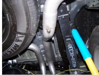
7. Install the passenger side overaxle tailpipe #F to the extension pipe. Use clamp #J to secure. Do not tighten. Insert welded hanger into rubber grommet.
