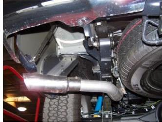
8. Install rear tailpipe hanger #K. Use bolt kit #L to secure. Use the hole on frame closest to the rear shackle. Install rubber grommet on rear hanger.
