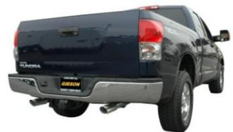
11. Install stainless steel tips. Clamp down. When you have everything in place, firmly tighten all bolts and clamps down securely. Use stainless steel cleaner and a Scotch Brite pad weekly to prevent tip from discoloration. Inspect all fasteners after 25-50 miles of operation and re-tighten as necessary.
