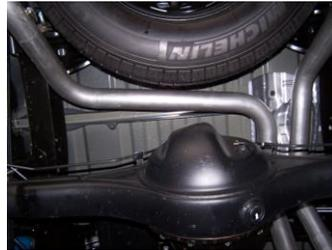
9. Install driver side overaxle tailpipe #G onto extension pipe, use clamp #J to secure pipe. Do not tighten. Insert welded hanger into rubber grommet.
