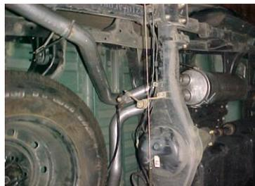
INSTALL PASS. SIDE TAILPIPE # D INTO MUFFLER 1-1/2" TO 2" USE CLAMP # I TO SECURE PIPE TO MUFFLER, DO NOT TIGHTEN. INSERT HANGER INTO RUBBER GROMMET.
