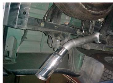
INSTALL EXIT PIPES # E ONTO TAILPIPES USE CLAMP # I TO SECURE PIPES TOGETHER. DO NOT TIGHTEN ON DRIVERS SIDE. USE CLAMP #I TO SECURE PIPE TO REAR HANGER #J.
