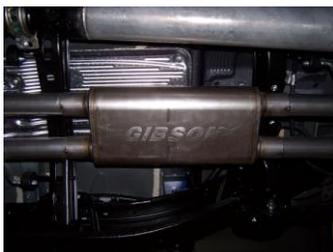
5. Install muffler #C onto headpipes 1.5"-2" with the louvers facing towards the converter. Use a jack stand to support the muffler. Use clamps #I to secure the muffler to the headpipes. Do not tighten. Muffler inlet is looking into the louvers.
