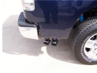
10. Install stainless steel tips. Clamp down. When you have everything in place, firmly tighten all bolts and clamps down securely. Use stainless steel cleaner and a Scotch Brite pad weekly to prevent tip from discoloration. Inspect all fasteners after 25-50 miles of operation and re-tighten as necessary.
