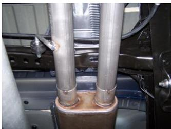
6. Install extension pipe #D into muffler. Use clamp #I to secure. Do not tighten. Next install driver side extension pipe #E into muffler using clamp #I to secure. Do not tighten. Insert welded hanger into rubber grommet.
