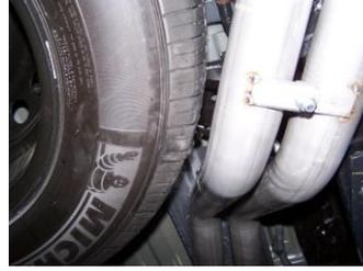
9. Use bolt kit #J to secure tabs. Make sure driver side tab is on the bottom. (You may need to loosen up the spare tire and move it over for better clearance.)
