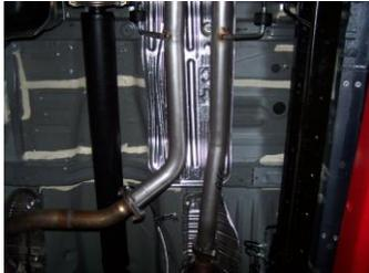
4. Install passenger side headpipe #A using your stock bolts. Do not tighten. Next, install driver side headpipe #B using stock bolts. Do not tighten. Install metal hangers into rubber grommets.
