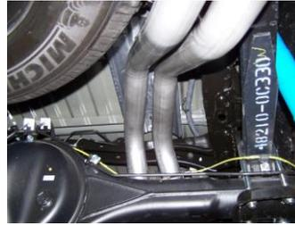
8. Install driver side overaxle tailpipe #G onto extension pipe. Use clamp #I to secure the pipe. Do not tighten.
