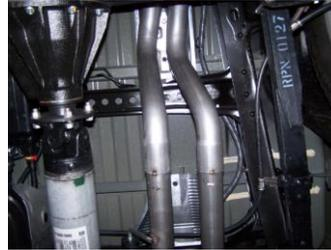
7. Install the passenger side overaxle tailpipe #F to the extension pipe 1.5"-2". Using clamp #I to secure pipes together. Do not tighten. Insert welded hanger into rubber grommet.
