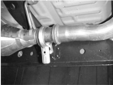
LAY OUT THE GIBSON EXHAUST ON THE FLOOR SO IT LOOKS LIKE THE DRAWING AND COMPARE PART NUMBERS. DISCONNECT THE FACTORY CLAMP IN FRONT OF THE STOCK MUFFLER AND REMOVE THE FACTORY EXHAUST. DO NOT DAMAGE THE FACTORY CLAMP. YOU WILL RE-USE IT. LEAVE
