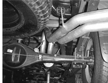
INSTALL THE DRIVERSIDE OVER AXLE TAILPIPE #D FROM THE REAR OF THE AXLE SLIP THE WELDED HANGERS INTO THE FACTORY RUBBER GROMMETS. THEN SLIP THE PIPE OVER THE OUTLET OF THE MUFFLER 1 1/2 TO 2". USE CLAMP # G TO SECURE TAILPIPES TO THE MUFFLER. DO NOT TIGHTEN.
