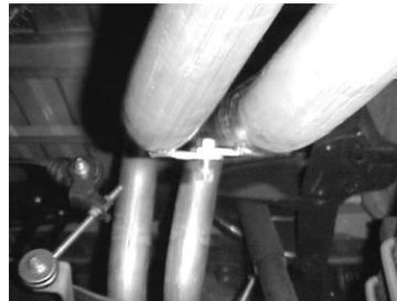
USING THE BOLT KIT # H, BOLT BOTH TAILPIPES TOGETHER. THE PASSENGER TAILPIPE MOUNTING BRACKET WILL BE POSITIONED ON TOP OF THE DRIVERSIDE TAILPIPE. ROTATE PIPE'S UNTIL YOU HAVE A MINIMUM OF A 1" CLEARANCE ON ALL PIPES FROM RUBBER BRAKE LINES, TIRES, SHOCK BOOTS, ETC.
