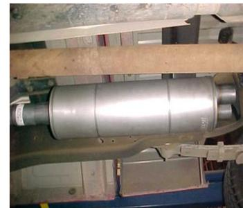
INSTALL MUFFLER AND ATTACH TO HEADPIPE. USING CLAMP #G. DO NOT TIGHTEN. USE JACKSTAND TO SUPPORT MUFFLER.
