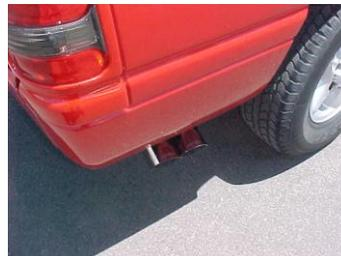
INSTALL THE STAINLESS TIPS. NOW GO BACK AND START AT THE FRONT AND TIGHTEN ALL CLAMPS AND HANGERS.
