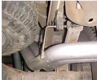
INSTALL PASSENGER OVERAXLE TAILPIPE #C. INSERT WELDED HANGER INTO RUBBER GROMMET. DO NOT TIGHTEN. ATTACH TAILPIPE TO THE MUFFLER USING CLAMP # F. USE BOLT KIT # I TO ATTACH BOTH OVERAXLE PIPES TOGETHER. THE SPARE TIRE ON SOME VEHICLES MAY NEED TO BE LOOSENED AND PULLED TO THE DRIVERSIDE FOR BETTER CLEARANCE.
