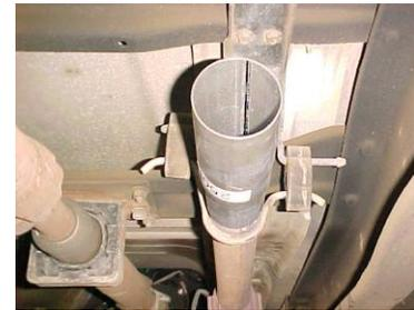
INSTALL HEADPIPE # A AND ATTACH TO THE STOCK EXTENSION PIPE USING CLAMP #F
