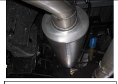
3. Install muffler #B onto headpipe 1.5" to 2" muffler outlets should be on top and level use clamp #G to secure together. Do not tighten. Insert hangers into rubber grommets
