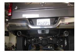
7.Install exit pipes #E onto tailpipes use clamp # F to secure together. After everything is installed begin to tighten all connections starting from the furthest forward connection. Items will move as you tighten. Be sure to check all clearance.
