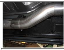
2.Install headpipe #A onto your factory pipe using clamp #G insert welded hanger into the rubber grommet leave clamp loose.
