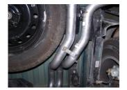
8. Attach tailpipes together with bolt kit #I. Do not tighten. Driver side tabs will be on the bottom.
