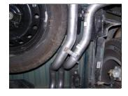
**7.** Attach tailpipes together with bolt kits #I. DO NOT TIGHTEN. Driver side tabs will be on bottom.
