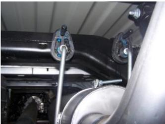
5. Slide band clamp #J onto muffler #B and attach with bolt kit #L. Do not tighten. Insert hangers into rubber grommets.
