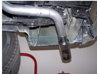
8. Install exit pipes #E onto tailpipes and secure with clamps #H. Do not tighten.
