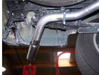
7. Install the driver side over axle tailpipe #D into the muffler 1.5-2". Use clamp #H to secure. Use another clamp #H to hold pipe up to hanger. Do not tighten. Insert welded hanger into rubber grommet.
