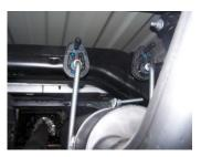
5. Slide band clamp #J onto muffler #B and attach with bolt kit #M. Do not tighten. Insert hangers into rubber grommets.
