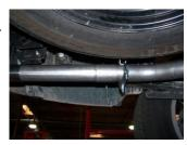
7. Install the driver side over axle tailpipe #D into the muffler 1.5-2". Use clamp #H to secure. Use another clamp #H to hold pipe up to hanger. Do not tighten. Insert welded hanger into rubber grommet.
