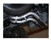
**7.** Attach tailpipes together with bolt kits #I. DO NOT TIGHTEN. Driver side tabs will be on bottom.
