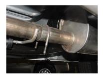
YOU MAY NEED TO HEAT IT UP FOR EASIER REMOVAL. LEAVE ALL RUBBER GROMMETS IN PLACE. USE WD-40 FOR REMOVAL OF HANGERS. FOR EASIER REMVAL, REMOVE THE TWO CROSSMENBER BARS FIRST.
