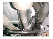
INSTALL HEADPIPE #A, YOU WILL NEED TO LINE UP THE TWO NOTCHES. INSERT WELDED HANGER INTO RUBBER GROMMET. USE CLAMP #H TO SECURE HEADPIPE TO THE STOCK PIPE. DO NOT TIGHTEN.
