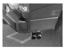
INSTALL THE STAINLESS TIPS. NOW GO BACK AND TIGHTEN ALL CLAMPS, NUTS AND BOLTS STARTING FROM THE FRONT AND WORKING BACK. TO CLEAN TIPS USE A SCOTCH BRITE PAD AND ANY STAINLESS CLEANER.
