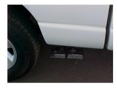
INSTALL YOUR STAINLESS TIPS. THERE IS A LEFT AND A RIGHT TIP. TIGHTEN ALL CLAMPS AFTER YOU MAKE SURE YOUR TAILPIPES ARE LEVEL.
