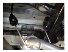
ASSEMBLY #A ONTO HEADPIPE 1-1/2" TO 2". SLIDE WELDED HANGERS INTO **RUBBER GROMMETS** YOU MAY NEED TO ADJUST WELDED HANGERS TO FIT INTO YOUR GROMMETS, USE A JACKSTAND TO SUPPORT YOUR MUFFLER. USE CLAMP #B TO SECURE IT TO YOUR HEADPIPE. DO NOT TIGHTEN.
