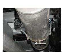
INSTALL MUFFLER #B ONTO HEADPIPE 1-1/2" TO 2". USE CLAMP #I TO SECURE THE MUFFLER TO THE HEADPIPE. DO NOT TIGHTEN. SLIDE BAND CLAMP #J ONTO THE MUFFLER AND INSERT THE WELDED HANGER INTO THE RUBBER GROMMET. ATTACH WITH BOLT KIT #L.
