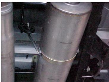
INSTALL MUFFLER #B ONTO HEADPIPE 1-1/2" TO 2". USE CLAMP #H TO SECURE THE MUFFLER TO THE HEADPIPE. DO NOT TIGHTEN. SLIDE BAND CLAMP #I ONTO THE MUFFLER AND INSERT THE WELDED HANGER INTO THE RUBBER GROMMET AND ATTACH WITH BOLT KIT #J.
