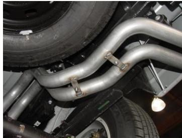
INSTALL PASSENGER SIDE TAILPIPE #D INTO MUFFLER AND ATTACH USING CLAMP #F. INSERT WELDED HANGER INTO RUBBER GROMMET. DO NOT TIGHTEN. USE BOLT KIT #I TO ATTACH THE TAILPIPES TOGETHER. DO NOT TIGHTEN. PASSENGER SIDE TABS ON TAILPIPE WILL BE ON TOP OF DRIVER SIDE TABS.
