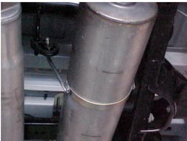
INSTALL MUFFLER #B ONTO HEADPIPE 1-1/2" TO 2". USE CLAMP #H TO SECURE THE MUFFLER TO THE HEADPIPE. DO NOT TIGHTEN. SLIDE BAND CLAMP #I ONTO THE MUFFLER AND INSERT THE WELDED HANGER INTO THE RUBBER GROMMET. ATTACH WITH BOLT KIT #L.
