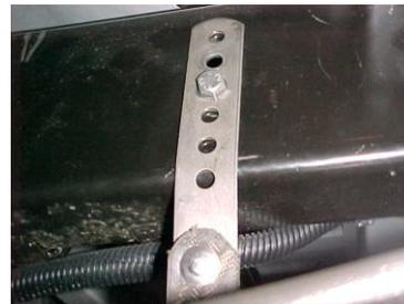
MEASURE 19 1/2" FROM THE REAR OF THE FRAME AND ON THE DRIVERS SIDE USE THIS HOLE AND BOLT ON HANGER #F. USE THE 3<sup>RD</sup> HOLE FROM THE TOP.
