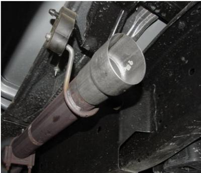
INSTALL HEADPIPE #A, LINE UP THE NOTCH USE CLAMP #D TO SECURE HEADPIPE TO YOUR FACTORY PIPE. DO NOT TIGHTEN.
