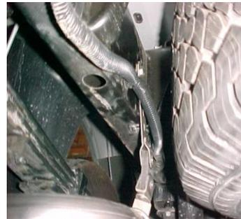
MEASURE 19 1/2" FROM THE REAR OF THE FRAME AND USE THIS HOLE AND BOLT ON HANGER #F. USE THE 1<sup>ST</sup>. HOLE FROM THE TOP. IT WILL BOLT ON THE INSIDE OF THE FRAME.
