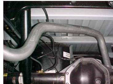
INSTALL THE EXIT PIPES #E ONTO THE TAILPIPES USING CLAMPS #G. ROLL THE PIPES UNTIL YOU HAVE THEM AT THE ANGLE YOU DESIRE.
