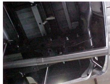
NOW GO BACK AND TIGHTEN ALL CLAMPS, NUTS AND BOLTS STARTING FROM THE FRONT AND WORKING BACK.
