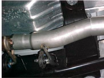
INSTALL HEADPIPE #A, YOU WILL NEED TO LINE UP THE TWO NOTCHES. INSERT WELDED HANGER INTO RUBBER GROMMET. USE CLAMP #A TO SECURE HEADPIPE TO THE STOCK PIPE. DO NOT TIGHTEN.
