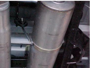
INSTALL MUFFLER #B ONTO HEADPIPE 1-1/2" TO 2". USE CLAMP #H TO SECURE THE MUFFLER TO THE HEADPIPE. INSERT WELDED HANGER INTO RUBBER GROMMET. DO NOT TIGHTEN. SLIDE BAND CLAMP #I ONTO THE MUFFLER AND INSERT THE WELDED HANGER INTO THE RUBBER GROMMET. ATTACH WITH BOLT KIT # J.
