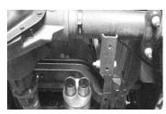
MAKE SURE YOU HAVE A 1" CLEARANCE ON ALL PIPES FROM BRAKE LINES, FUEL LINES, SHOCKS, TIRES, ETC...
