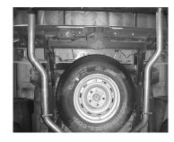
OVERAXLE TAILPIPE # C 1-1/2" TO 2" FROM BEHIND THE AXLE AND CONNECT TO THE MUFFLER AND ATTACH WITH CLAMP **#F. INSERT WELDED** HANGER INTO RUBBER GROMMET. ATTACH HANGER #H USING CLAMP #F TO TAILPIPE. REPEAT THE SAME FOR THE DRIVERSIDE OVERAXLE TAILPILPE # D. IF YOU CAN NOT GET THE PASSENGER TAILPIPE TO CLEAR REMOVE SPARE TIRE AND ROTATE THE MUFFLER TOWARDS THE DRIVERSIDE AND ALIGN TAILPIPES
