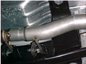
INSTALL HEADPIPE #A ONTO YOUR EXISTING STOCK FRONT PIPE AND SECURE WITH CLAMP #F. USE A JACKSTAND TO SUPPORT THE CONVERTER. INSERT WELDED HANGER INTO RUBBER GROMMET.
